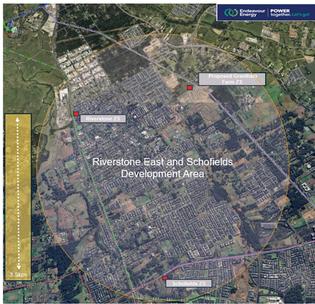
Figure 13 – Riverstone East and Schofields development area in relation to existing and proposed network assets
