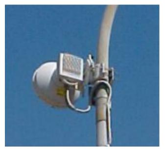
Parabolic Dish type antenna
