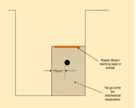
Figure 5 – Cable excavation clearances
