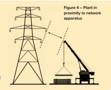
When loading or unloading equipment using plant, great care shall be taken to ensure that no part of it, or its load, comes within the safe approach distance relevant to the voltage concerned.
