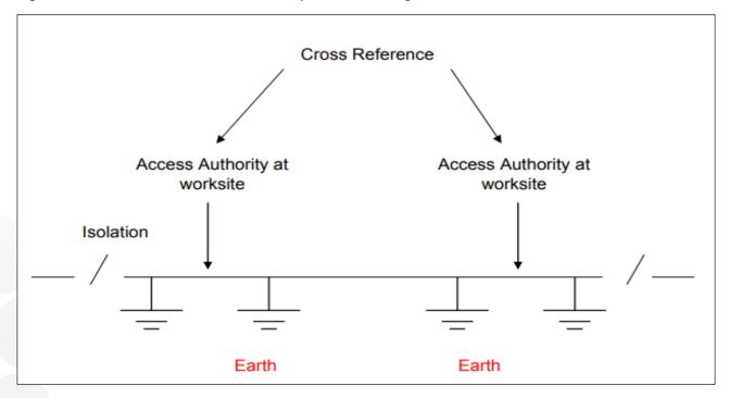
Figure 31 – Cross referenced AAs with common earthing for each worksite
