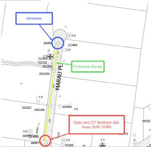
Figure 25 – Example of worksite with no network mains beyond
