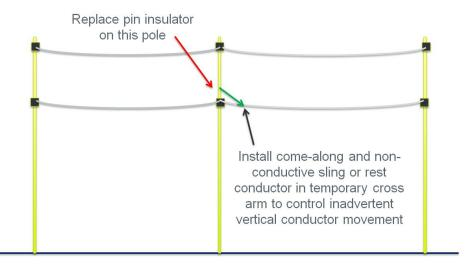
Note: Confirm all come-alongs/ratchet pullers/service strainers/slings and stockings are of the correct type and size to allow the job to be completed safely.
