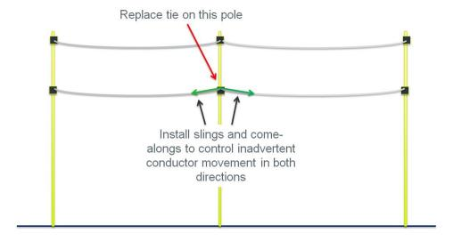
Where a small amount of tension is required to be taken up in a conductor to complete the task (for example, replacement of a cross arm or an insulator) secure the conductor being worked on in both directions (that is, on both sides of the structure) with come-alongs and ratchet pullers to restrain conductors, as shown in Figure B, before commencing the task.
