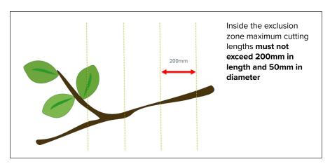
The cut and hold technique may only be used if there is no possibility to make contact with the network i.e. a clear line of site directly below. Any vegetation trimming directly above the mains shall be no more than 50mm in diameter or 200mm in length. A drop zone shall be nominated, established and noted prior to using the cut and hold technique, the established drop zones shall have a clear line of site and free of mains at all times.
