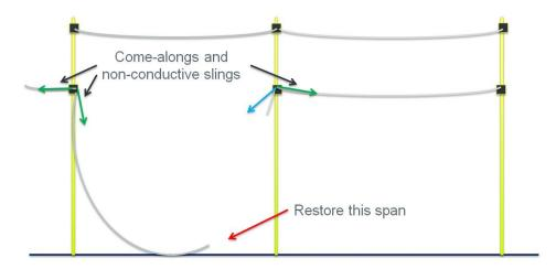
**At the structure where the work is occurring,** secure the conductor being reinstated with a come-along and ratchet puller to restrain and control the tension in the conductor.
