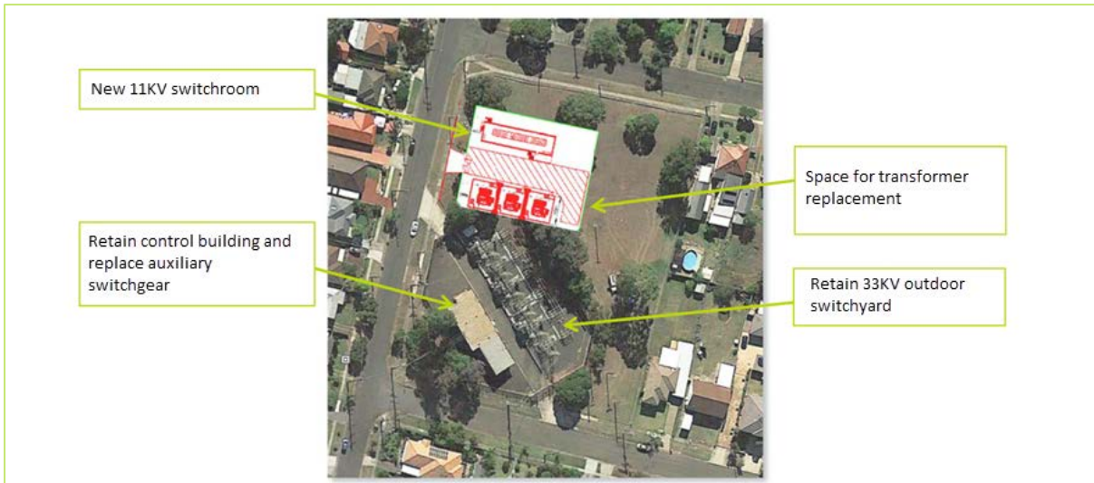
Figure 9: Marayong ZS Renewal Option B – new 11kV switchroom building to the north of the existing ZS.
