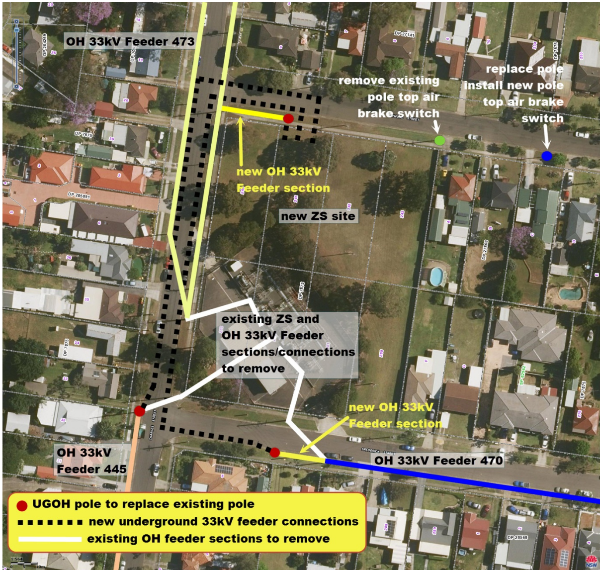
Figure 3: Marayong ZS redevelopment - associated feeder design.
