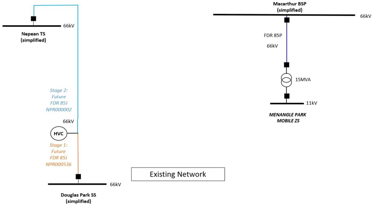
The Menangle Park mobile substation has a single transformer with a total capacity of 15MVA. If there is a failure of the 15MVA transformer or a failure on the 66kV transmission feeder 85P then there is only a firm backup capacity of 5.67MVA from the adjacent zone substations via feeders NN1251 and T874.
