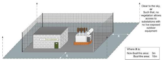
Figure 22: Clearances required around and above a Substation (Source: Endeavour Energy's MMI 0013)
