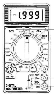
Turn the meter to the DCV quadrant depending on your voltage supply. Start at 20V then work down through the dial until you get a reading that makes sense on the display. Remember 2000 m is representing 2000 millivolts or 2V while 200 m is measuring 0.2V. Most batteries are 1.5V.
